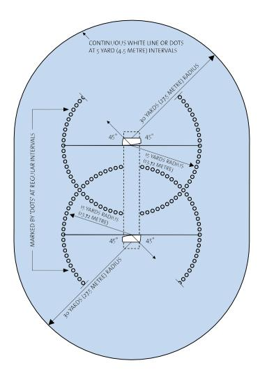
The final mark of the 15 yards radius shall be a line placed at an angle of  $45^\circ$ , measured from the popping crease at a point level with the middle stump.
